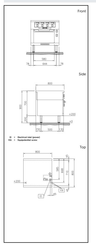
Modular Cooking Range Line thermaline 80 - Electric Free-cooking Top on Oven H=700
